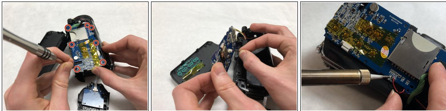
*(i)* Although it requires extra steps, it is advised that you remove the motherboard and screen to ensure that nothing is damaged in the process of replacing the lens.
