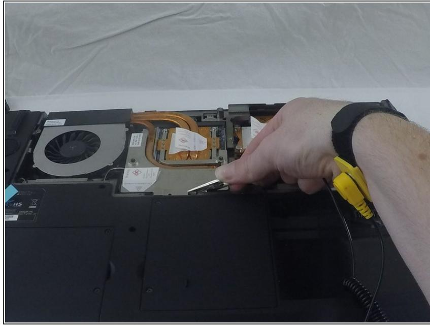
**⚠** An electrostatic discharge could damage your computer. Use an electrostatic wrist strap when working inside the computer.
