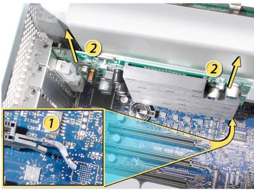
⚠ Handle the card only by the edges. Do not touch its connectors or any of the components. Lift the card straight out from the connector to remove it, and insert it straight into the connector to install it. Do not rock the card from side to side and don't force the card into the slot. Once the replacement card is installed, pull on it gently to check.
