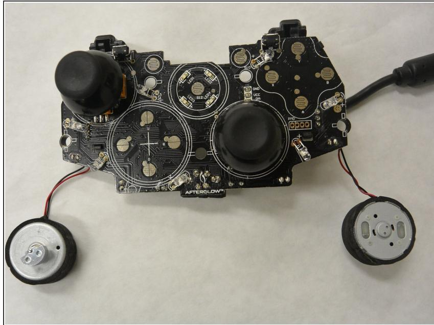
*(i)* The rumble motors are located in the bottom right and left hand corners of the controller.
