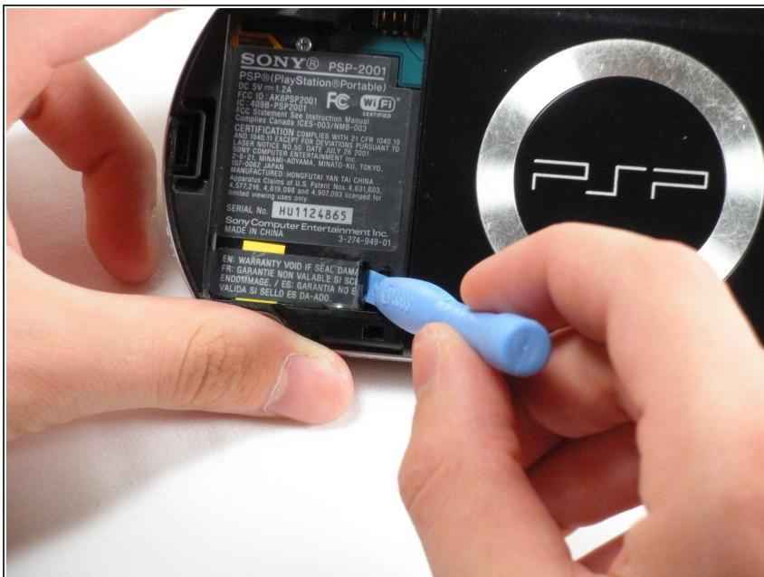
**⚠** This step requires the removal of the warranty sticker. **Removing the sticker will void the warranty.** According to the FTC removing this will not void your warranty.
