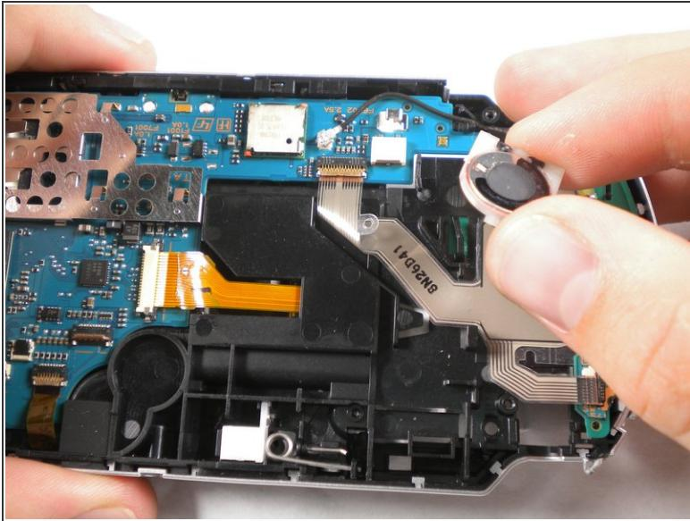
**⚠** Push the black tab at the bottom of the speaker to pop the speaker out of place, and remove the speaker.
