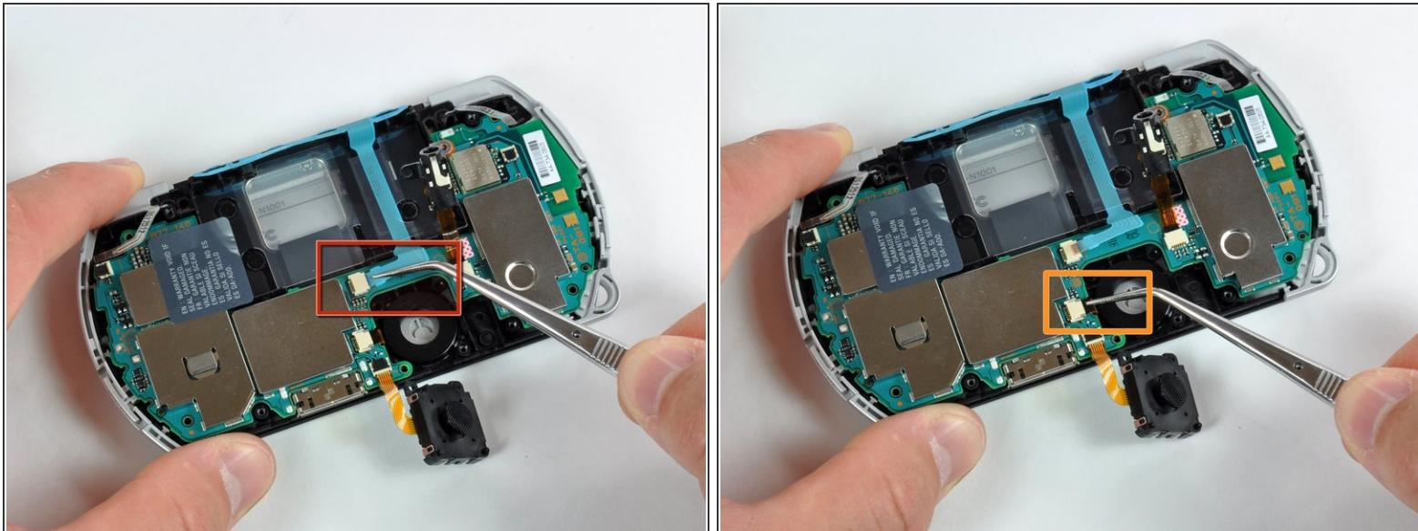
**⚠** Be very careful when disconnecting the following cables. The connectors do not have flip-up tabs; just hold each cable steady and pull it out of the connector.
