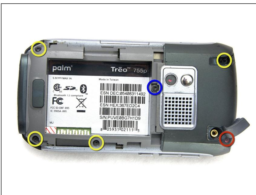
**⚠** **WARNING:** The top right red screw marked by the red circle has a warranty seal. Removing this seal will void your warranty.
