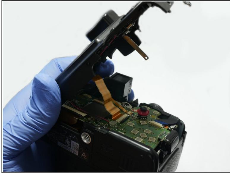
**⚠** Please be careful. Do not lift the cover fully because it is still attached to the Main Board via flex cables.
