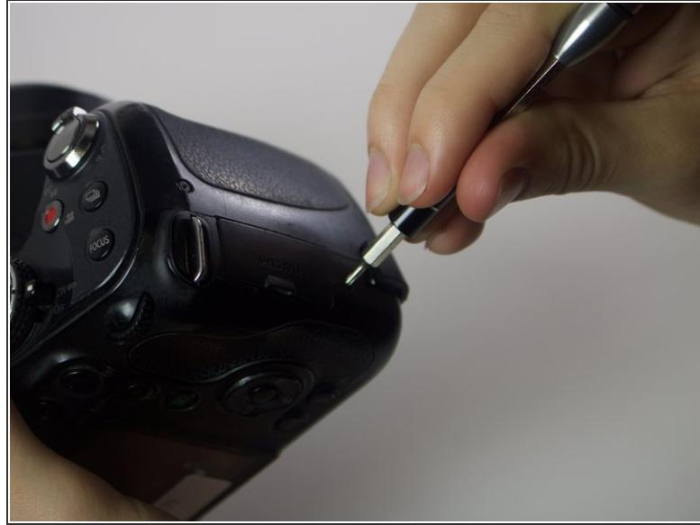
*(i)* All screws should be removed using a Phillips #0 screwdriver.
