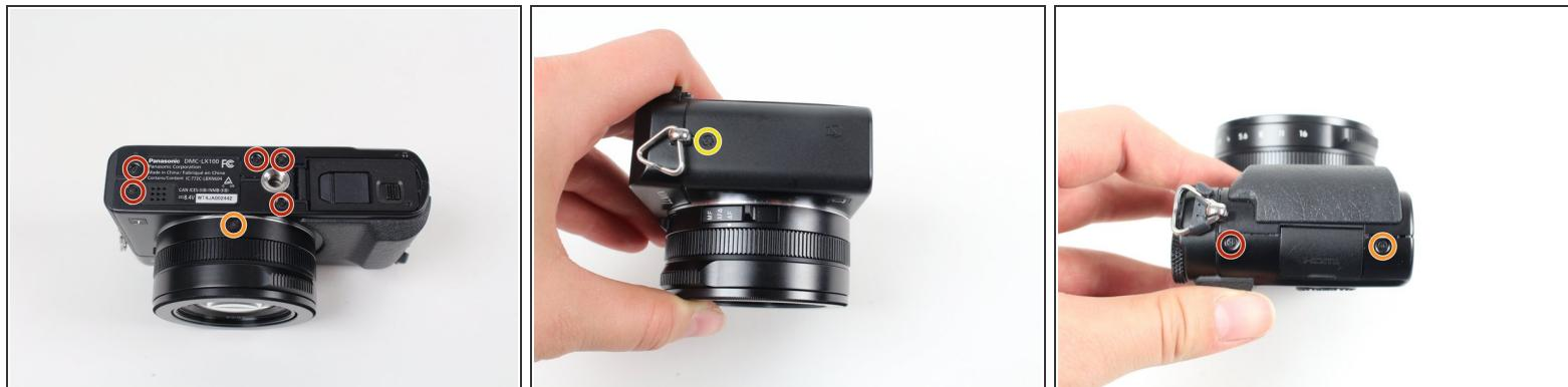
⚠ Some of these screws may have adhesive to keep the camera from being taken apart so push hard with the screwdriver and turn slowly to avoid stripping screws.
