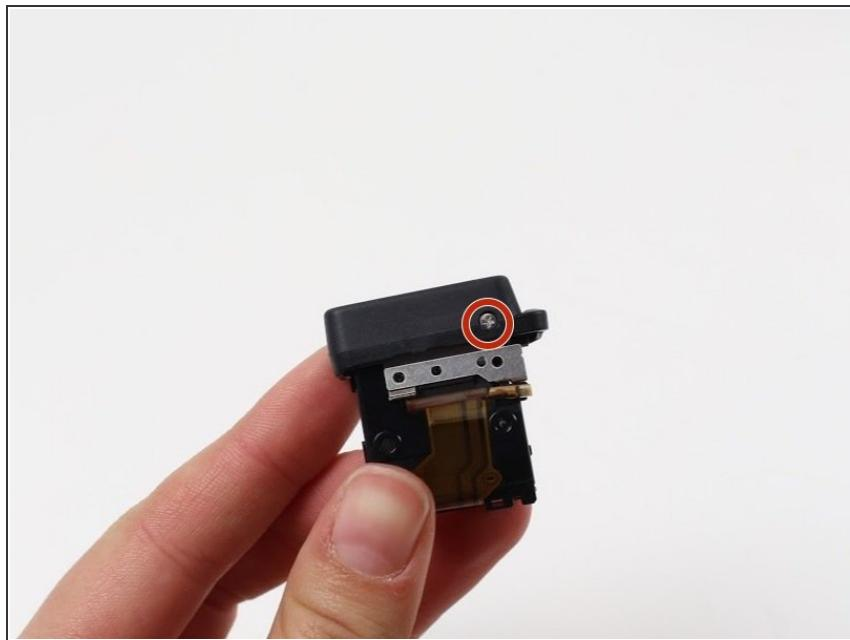
**i** The viewfinder in this picture is taken off of the camera to more easily see where the screw is located. It is not actually removed from the camera.
