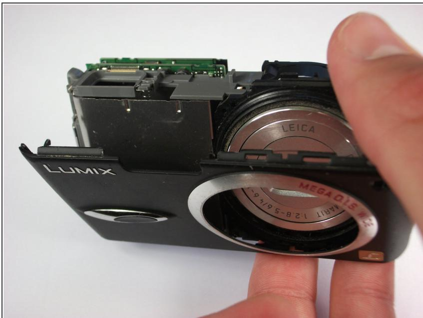
⚠ Carefully remove the front casing after verifying that the thin plastic around the lens is not still attached.
