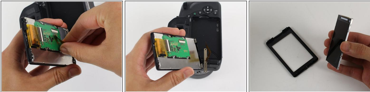
**⚠** Do not yank out the electronic ribbon attached to the screen and the screen mount, or you may damage it. To properly detach this ZIF connector ribbon, see [this technique on disconnecting ZIF connectors](#).
