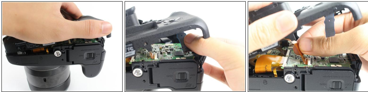
**⚠** Do not yank off the back plate. If you do, you will tear the electronic ribbons attached to the inside of the camera and the back plate.
