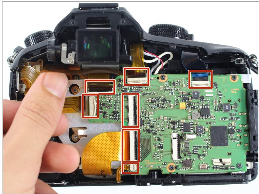
**⚠** Do not yank out the electronic ribbons attached to the motherboard, or you may damage them. To properly detach these ZIF connector ribbons, see [this technique on disconnecting ZIF connectors](#).
