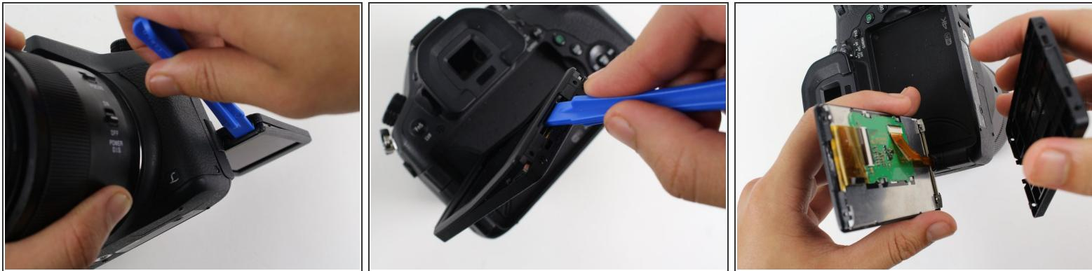
**⚠** In this step you will pry off the two sides of the screen's plastic casing. Do not yank off the side that holds the glass screen. If you do, you will tear the electronic ribbon attached to the screen and the screen axle.
