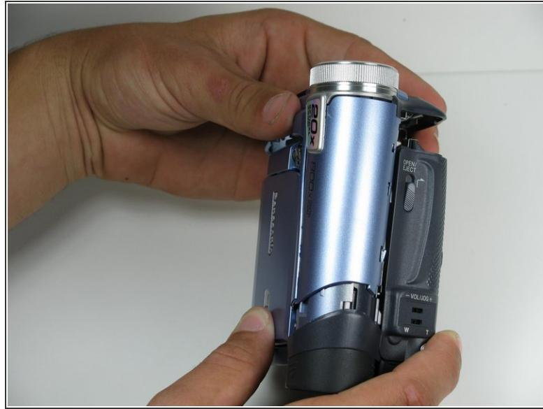
**⚠** Very carefully remove the front cover from the main body of the camcorder.
