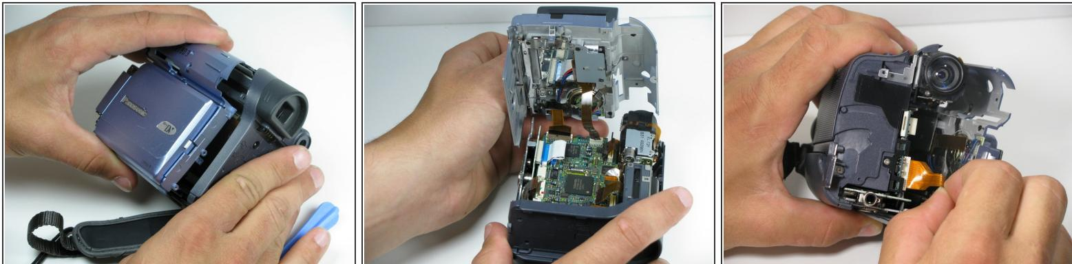
! Before removing the LCD panel from the camcorder, disconnect the ribbon cables joining the LCD panel to the logic board.
