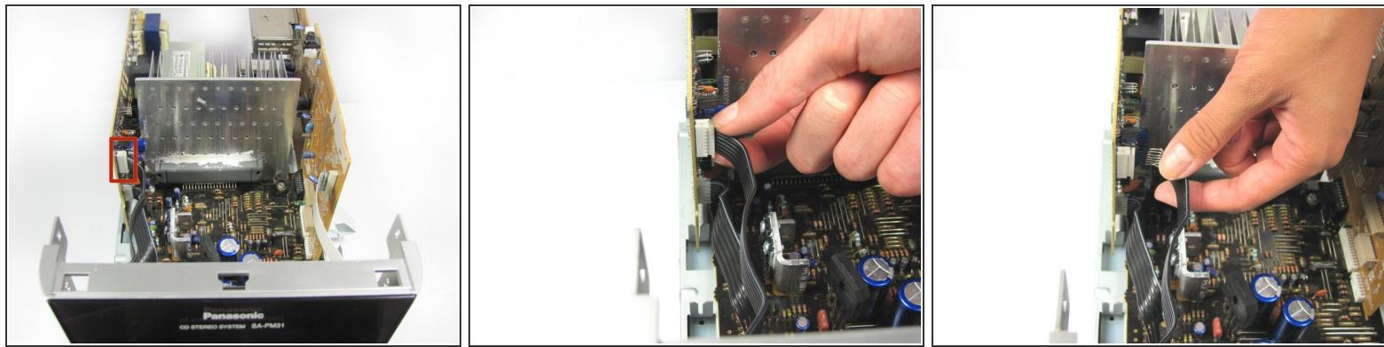
**!** Unlike the other ribbon wire connectors, the white connector (in this step only) is not attached to the ribbon wire. It can not, and should not, be pulled out completely.
