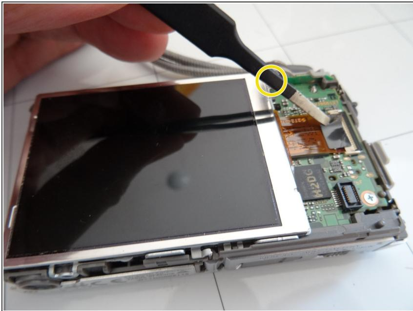
⚠ Under the gray plastic molding you will find the motherboard. You do not have to replace the ribbon cable to the display. It is enough to fold the display away!
