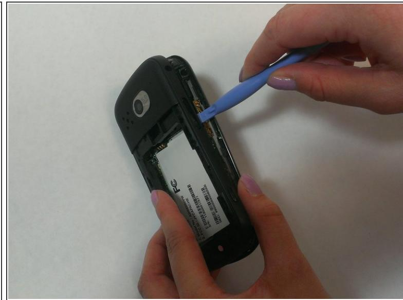
**⚠** Be careful when prying the plastic bezel and back case apart from each other; the parts are connected by both snaps and adhesive. Forcing the back case off could result in it breaking or cracking.
