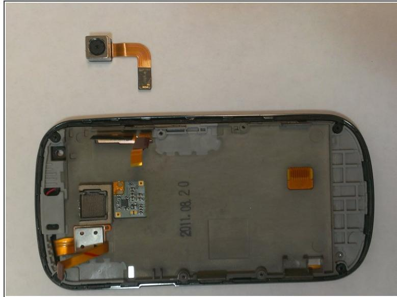
*(i)* The rear facing camera is attached to the back of the screen with adhesive.
