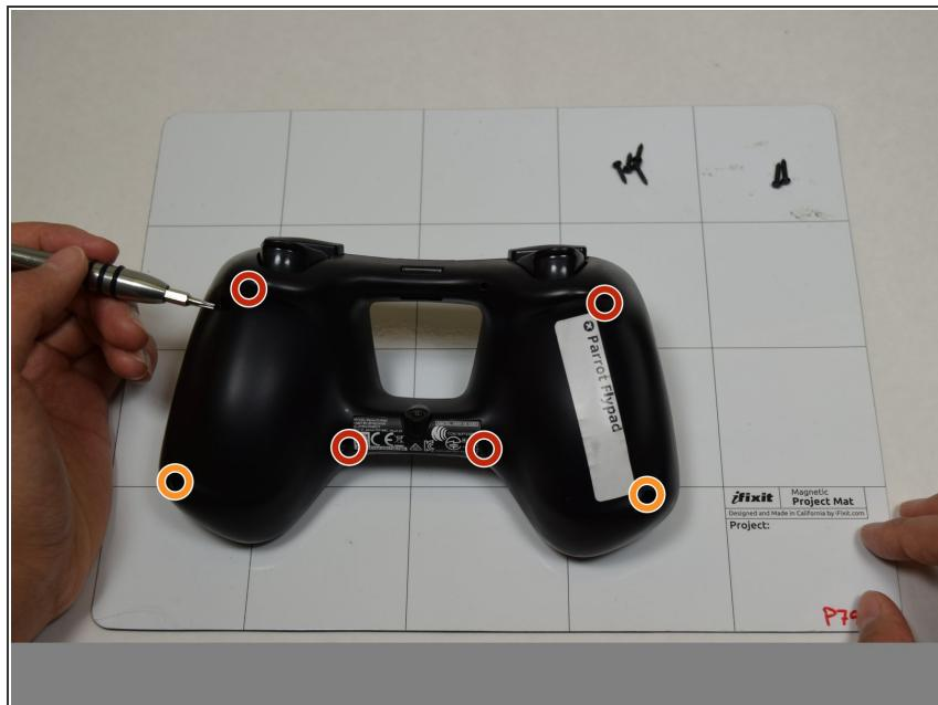
**i** Total of 6 Screws are located in the back of the controller.
