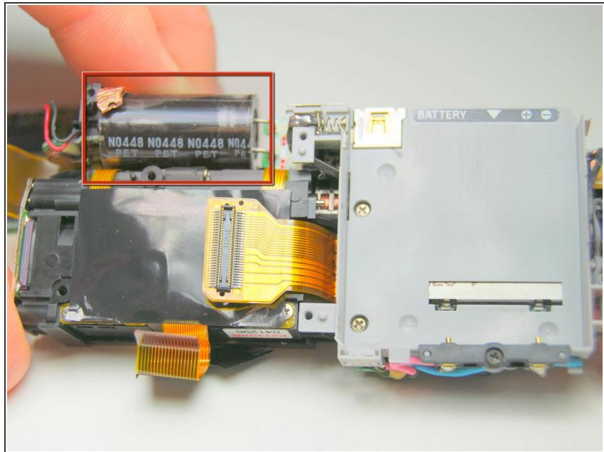
**⚠** Do not touch the black cylinder on the top edge. This is the capacitor for the flash and it may shock you.
