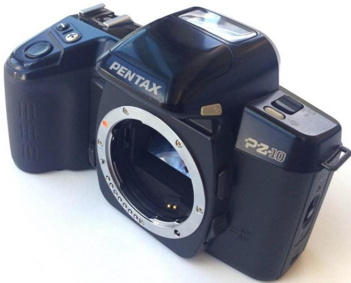
ⓘ The top cover is one piece encasing the top of the device except the shutter release button and flash.
