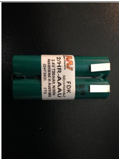
**i** Finding a battery is tough. I'm not sure which ones work. This one specially made up by BatteryWorld (Melbourne Australia) for \$26 FAILED later. If you find a better solution let me know.
