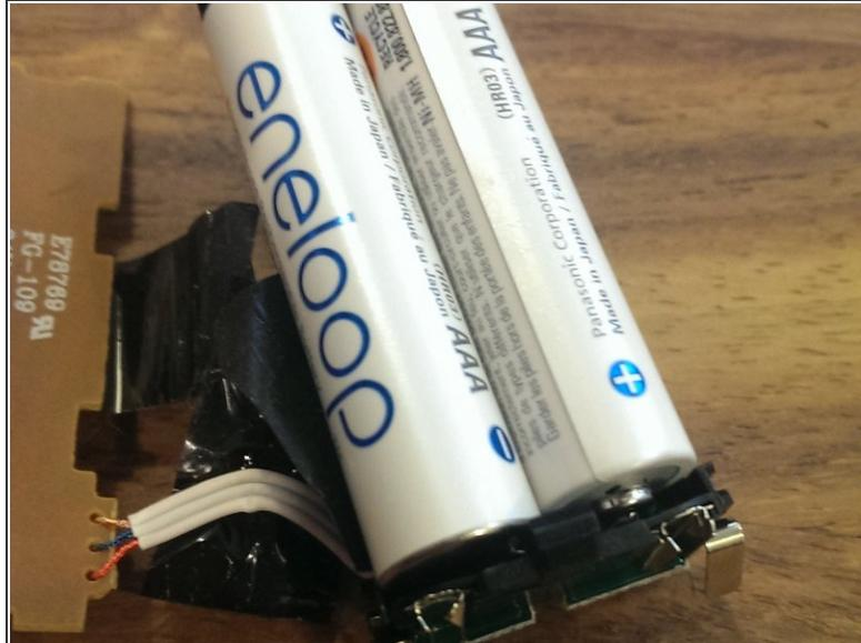
**⚠** Replacing the batteries is difficult. **The wires must be as in this picture** - there is simply no room for them to be anywhere on the outside of the housing.
