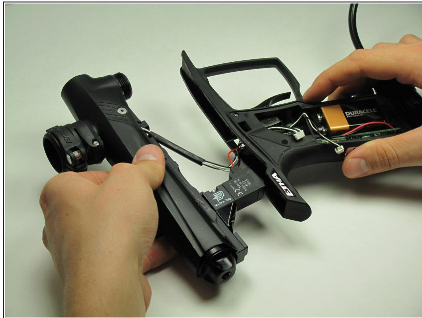
**⚠** Be very careful during the step to avoid damage to the solenoid or wiring.
