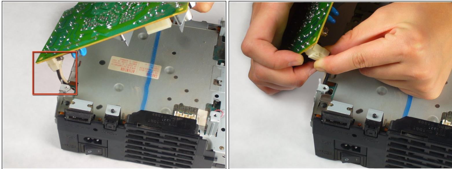
**⚠** Do not remove the power board yet. It is still attached to the motherboard assembly via the power board connector (highlighted in the first picture), which is located next to the main power switch.
