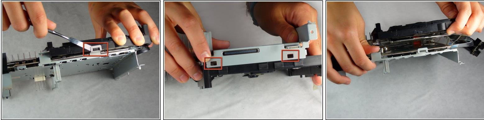
ⓘ Unclip flaps, one on one side and two on the other, holding the disc drive together. **The first two pictures display where the three flaps are.** This is very tricky so take your time.
