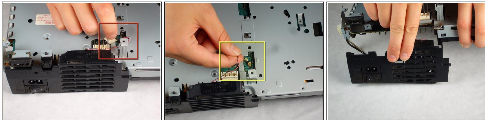
*(i)* We can now remove the fan and main power switch assembly.
