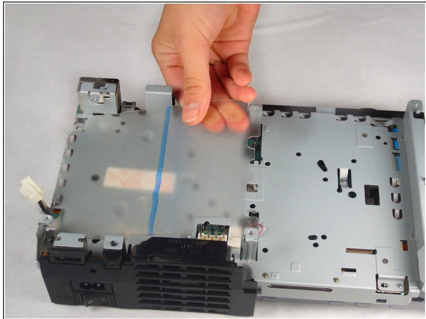
*(i)* The transparent piece of plastic located underneath the power supply recess in the motherboard assembly is the heat shield.
