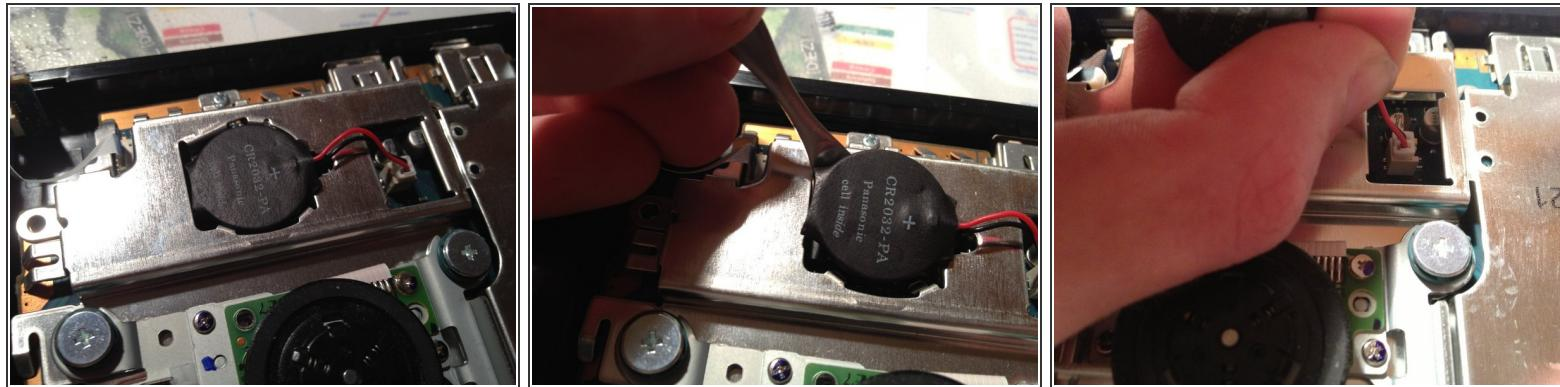
**(i) Locate the battery on the motherboard**
