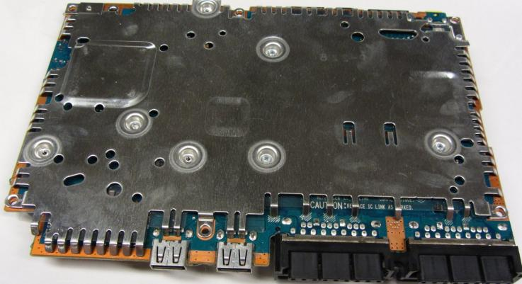
*i* Take the motherboard and flip it upside down. On the back of the motherboard, you should locate another metal plate that is attached to the back of the motherboard.
