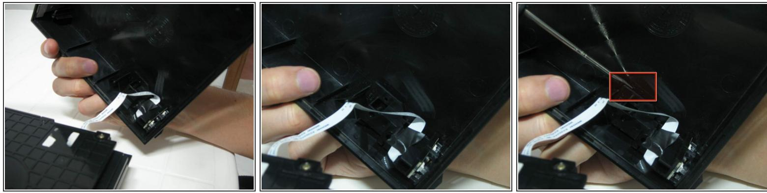
⚠ This model has a flat cable to the reset and eject button. Take extreme caution to not destroy it.
