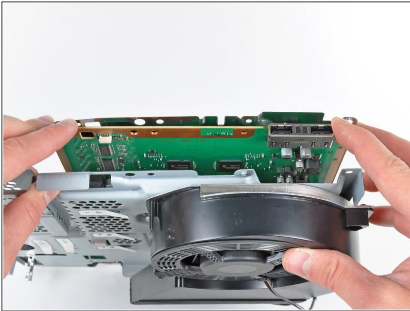
*(i)* If necessary, gently pry the motherboard off the top shield near the heat sink and its shroud.
