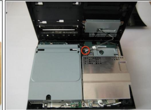
**⚠ READ THIS ENTIRE STEP AND THE NEXT ONE BEFORE PROCEEDING.** Locate the two locking tabs on the back of the PS3. Push them in simultaneously and lift the outer plastic shell off of the main board but BE CAREFUL as there is a ribbon cable connecting the shell to other hardware.
