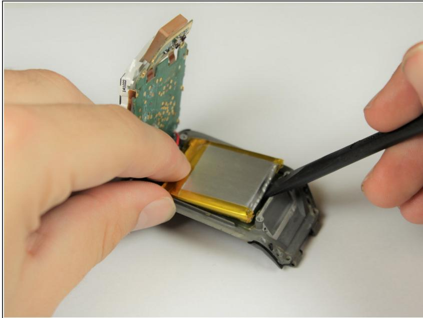
**i** The battery is glued down to the back of the watch. It may take some force to detach the battery at the glue joint.
