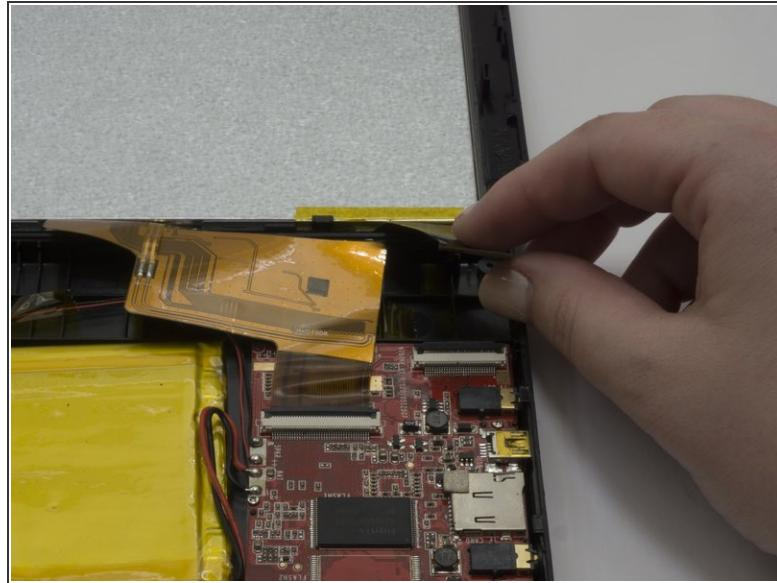
i The flexible flat cables (FFC) attach to parts in the bottom panel with zero insertion force (ZIF) connectors.
