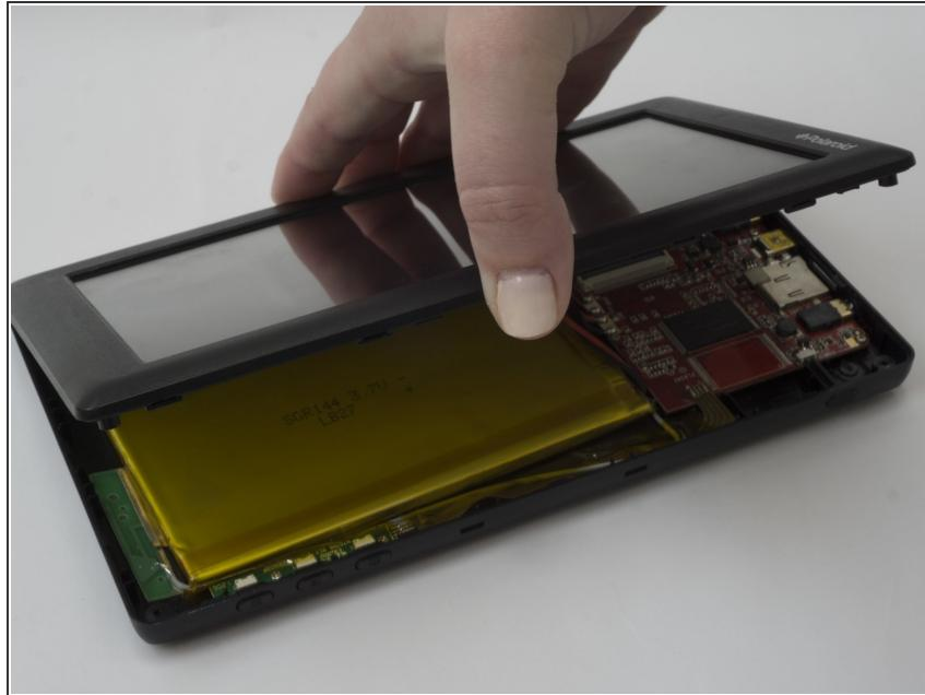
! Removing the panel too quickly may damage the cable that attaches parts between the two panels.
