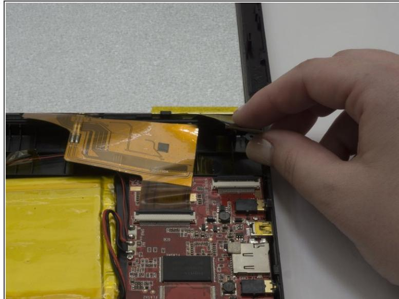
ⓘ The flexible flat cables (FFC) attach to parts in the bottom panel with zero insertion force (ZIF) connectors.
