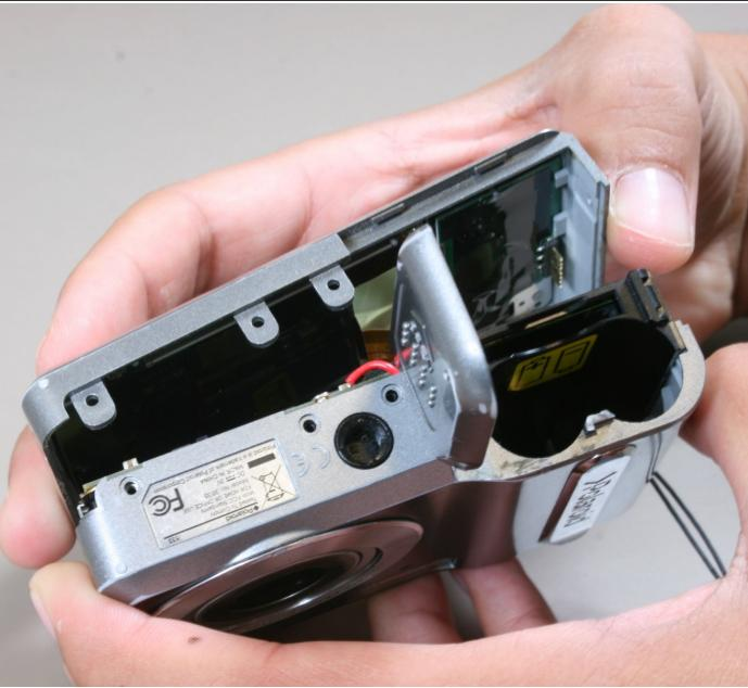
**⚠** Be careful not to pull the cover off completely, as it should remain attached to the motherboard.
