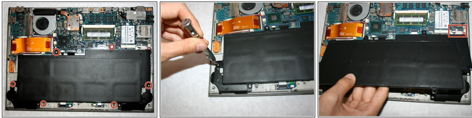
**i** The battery is the black rectangular piece in the bottom half of the device.
