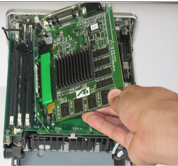
! Carefully lift the video card from the logic board.
