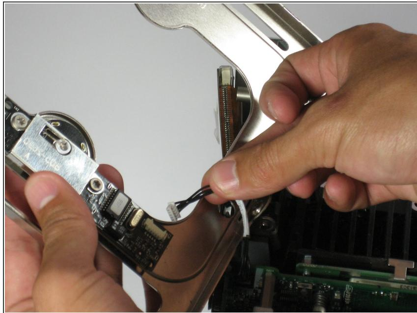
**⚠** Slowly lift the plate off the cube and disconnect the power cord.
