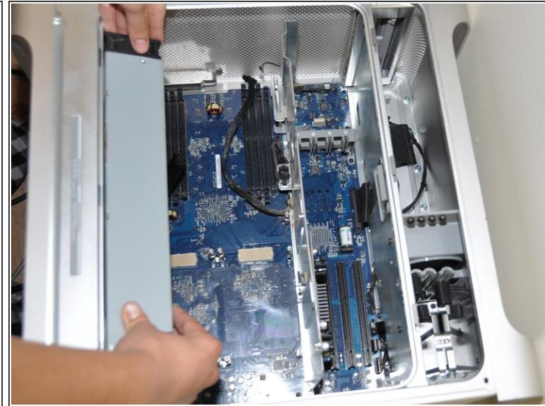
**ⓘ** Carefully pull the power supply out of the case.
