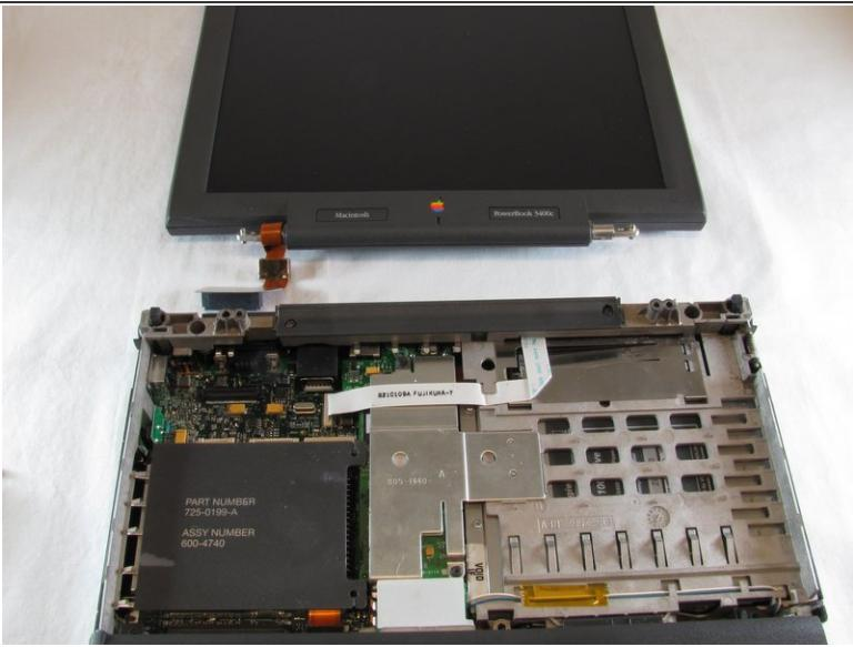
**⚠** The two T8 13 mm torx screws hold the display screen in place. Be sure to remove the screws while supporting the screen or else it will fall.
