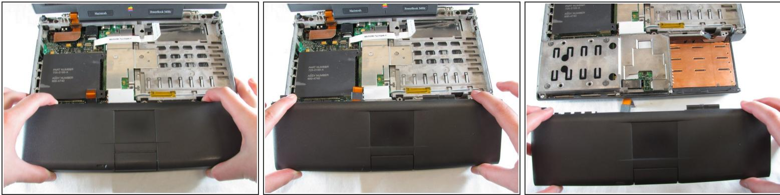
**⚠ WARNING:** There is a high risk of breaking the tabs that lock the panel to the casing. Remove the panel slowly and cautiously to avoid damage.
