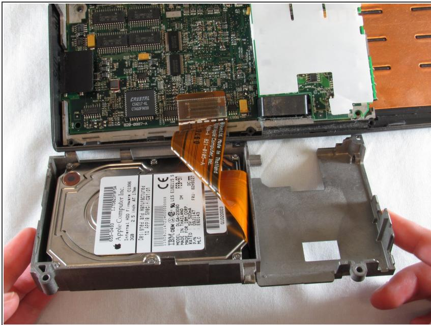
⚠ A ribbon cable is attached to the underside of the hard drive. Hasty removal of the hard drive can damage the ribbon cable.
