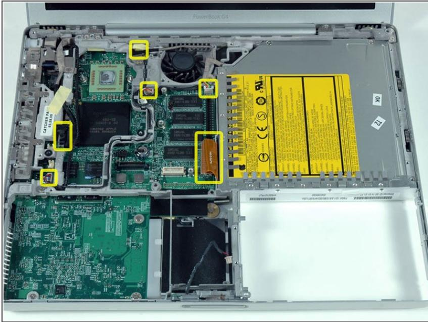
**⚠** The connectors at the ends of the cables are often attached very firmly to the sockets on the logic board. Pulling directly on the cable will either separate the cable from its connector or the socket from the logic board.
