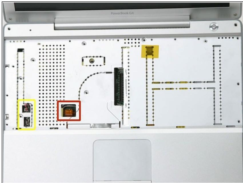
**⚠** This step is extremely tricky, and has the potential to ruin your computer. It is easy to pull the plug with the red and black leads (the power) out of the motherboard. If you do that, it is nearly impossible to fix.
