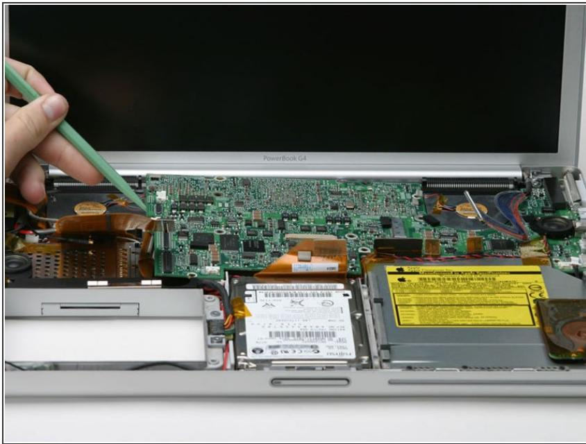
**i** Two cables still connect to the logic board and must be removed before pulling the board entirely out of the computer.
