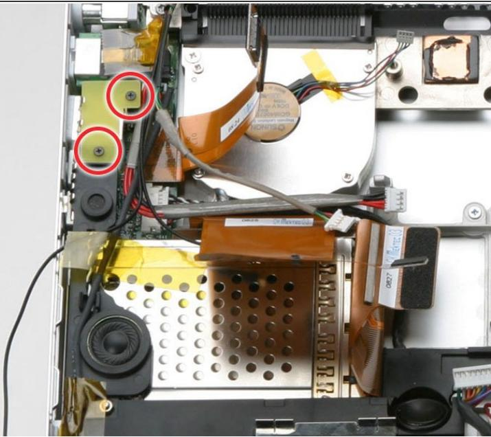
On computers with an ambient light sensor, you will remove an ambient light sensor board instead of a placeholder yellow plastic board.
