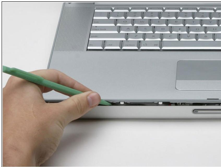
**i** There is one latch that stops you from pulling the upper case right off, located on the left side of the optical drive slit. To free the upper case, you will be pulling a thin metal latch toward you, freeing it from the clasp holding it in place.
