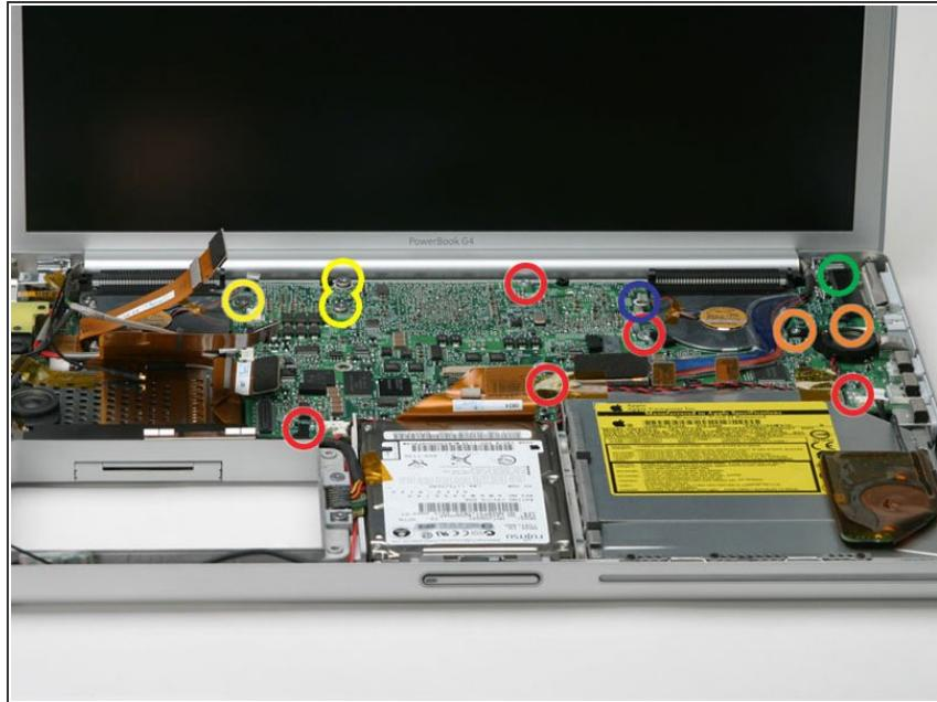
**ⓘ** There should be no cables connected to the top of the logic board at this point.
