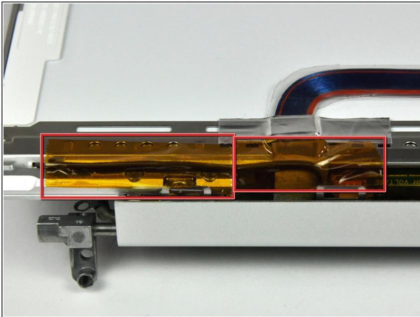
ⓘ If necessary, remove the two pieces of tape covering the inverter leads.
