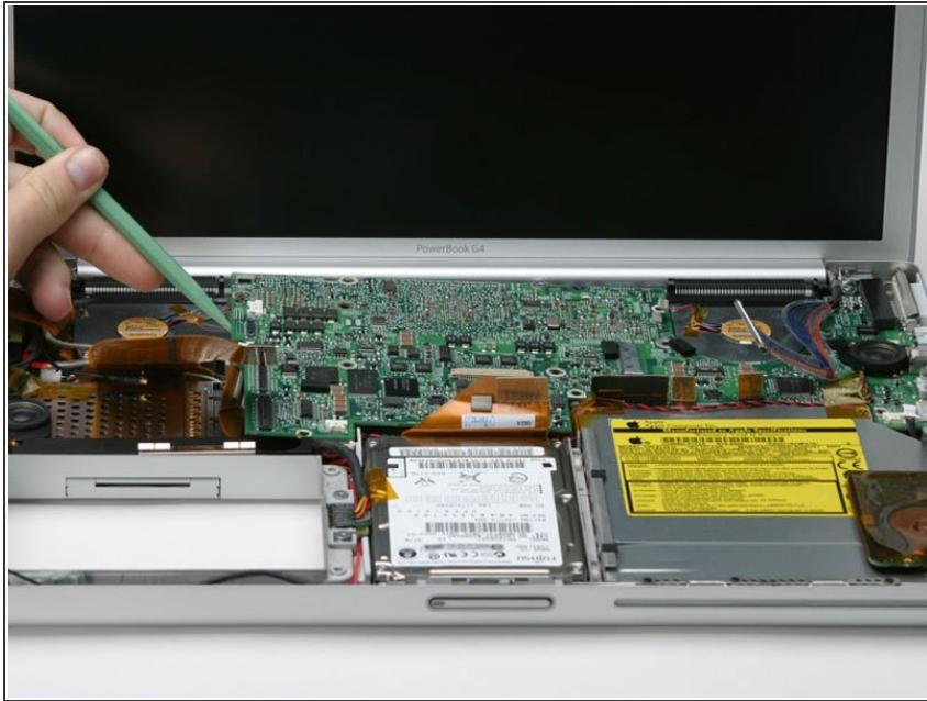
**ⓘ** Two cables still connect to the logic board and must be removed before pulling the board entirely out of the computer.
